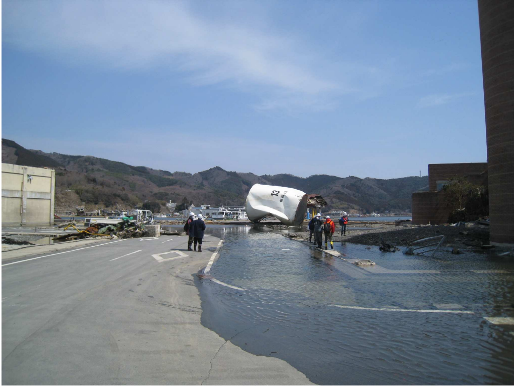
Figure 3 Ground settlement causing submerged land by sea water
