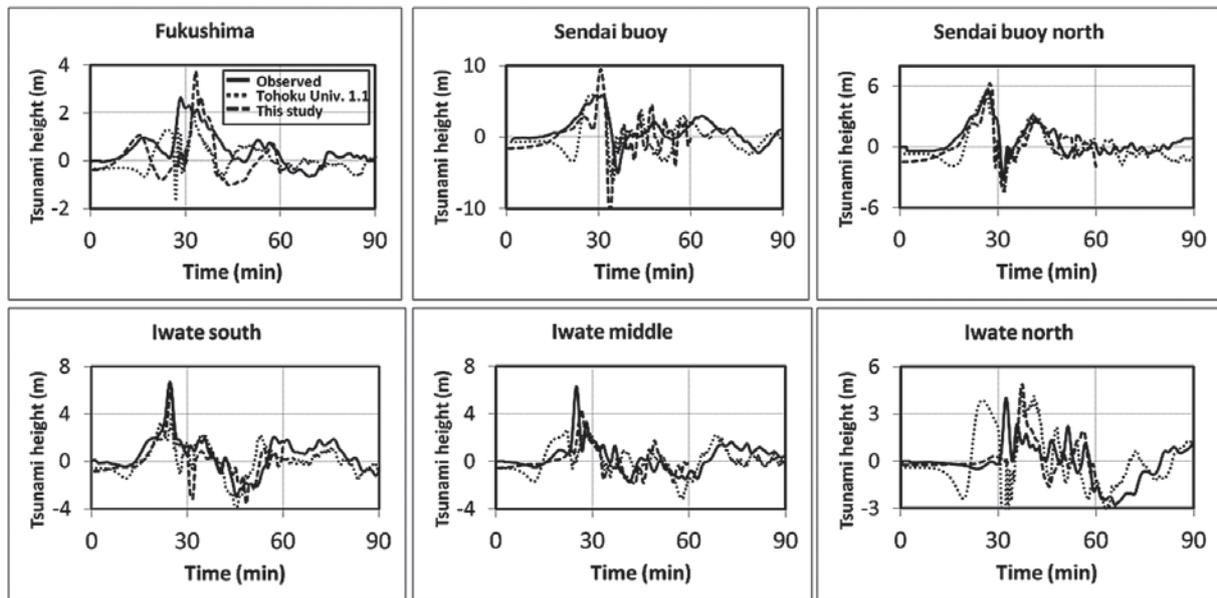
**Figure 5.** Comparison of the observed tsunami waveforms with the modeled tsunami based on the source model of Tohoku Univ. 1.1 and source model proposed by this study
