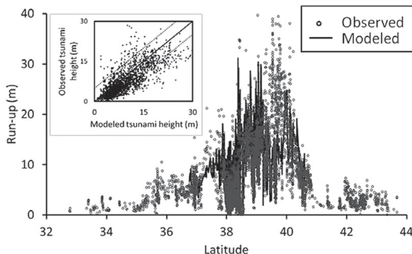
Figure 4. Comparison of modeled run-up heights based on Tohoku Univ. 1.1 model with the observed data
