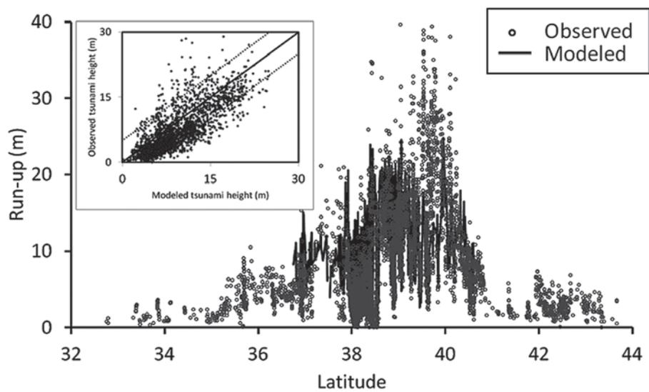
Figure 8. Comparison of modeled run-up heights using the proposed source model with the observed data
