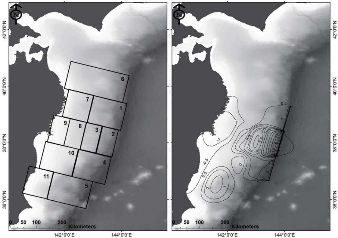
**Figure 6.** Fault segments representing the 2011 rupture area (left), and the resulting calculated sea-floor displacement (right).
