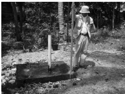
Photo 3.3.2.2 Bench mark of Bench 1 at Lale The reference point is at the intersection point between the staff and concrete base.
