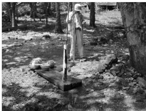
Photo 3.3.2.3 Bench mark of Bench 2 at Lale The reference point is at the intersection point between the staff and concrete base.
