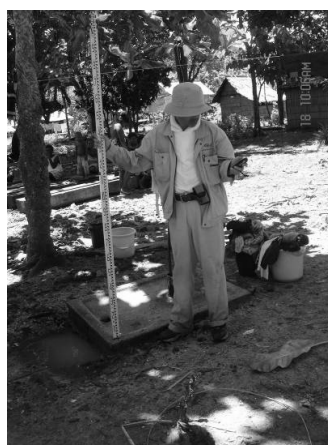
Photo 3.4.7.2 Bench mark of Bench 7 at Varese The reference point is at the intersection point between the staff and concrete base.
