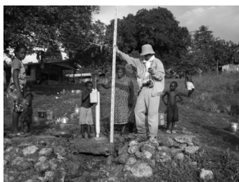
Photo 3.3.8.4 Bench mark of Bench 3 at Koriovuku. The reference point is at the intersection point between the staff and concrete base.
