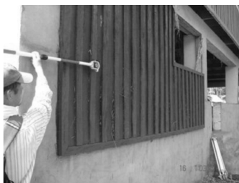
Photo 3.2.6.2 A line of water mark of scratches was traced on the wall of the centenary hall in Lengana.
