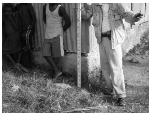
Photo 3.3.8.5 Bench mark of Bench 4 at Koriovuku. The reference point is at the intersection point between the staff and concrete base.
