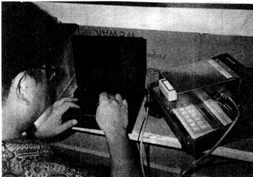
Photo 2 Installing the seismic records with ground acceralation sensors in three components
