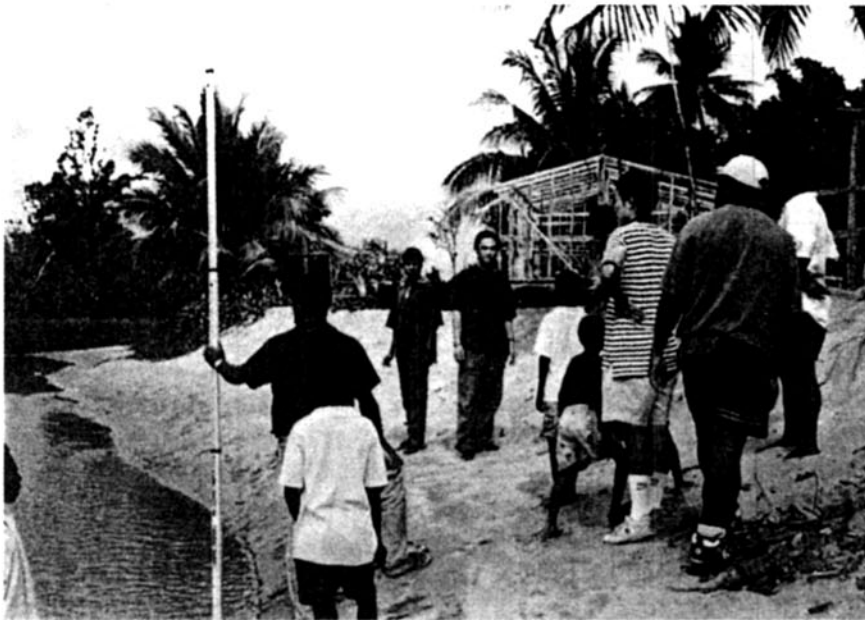
Photo 1 Survey team on the coast measuring tsunami heights after interview and checking marks
