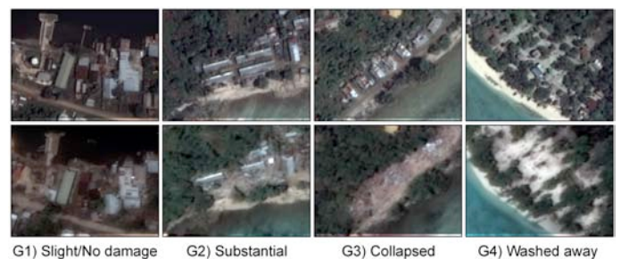
Figure 8. Damage classification from pre and post event imageries.
